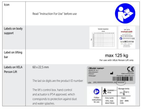
Labels on the lift should be read at a distance of approx. 40 cm under normal daylight conditions.
